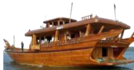
The Beypore Uru is a traditional dhow that was built in Beypore, India, with a legacy that dates back to the 11th century. Made from pure Malabar teak and coir, these vessels have been used for generations to facilitate trade, and are renowned for their unique design and skilled craftsmanship.
